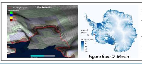
BISICLES-computed simulation of present-day Antarctic ice velocities. The image at the left illustrates adaptive placement of fine spatial resolution near grounding lines (red) for the Pine Island Glacier.
