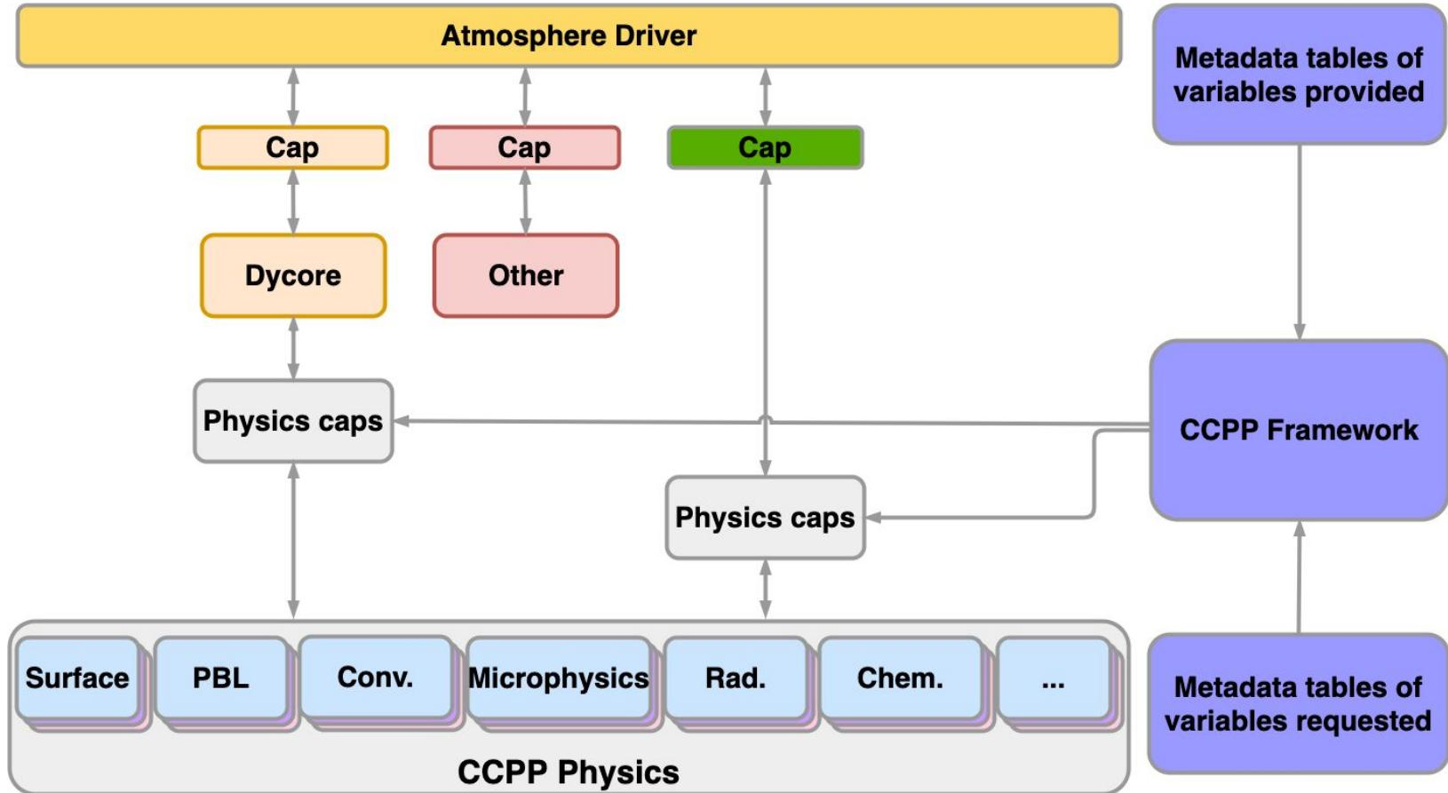
The CCPP is a software framework that automatically generates the Fortran interface (cap) layer for a physics parameterization (scheme).
