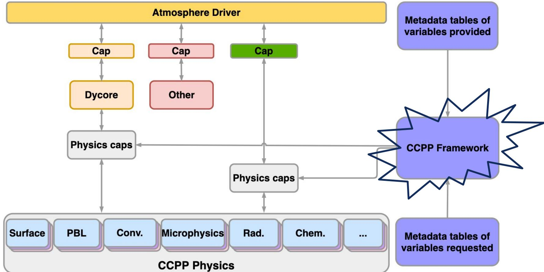
The CCPP is a software framework that automatically generates the Fortran interface (cap) layer for a physics parameterization (scheme).
