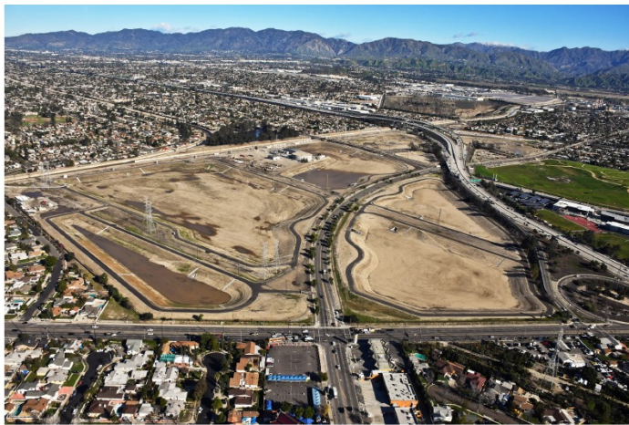
Los Angeles' Tujunga Spreading Grounds collect stormwater and let it percolate into the earth. Such "sponge city" projects are changing urbanites' relationship with water. COURTESY OF LOS ANGELES DEPARTMENT OF WATER AND POWER
