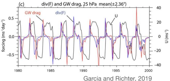
Contributions to the zonal-mean acceleration from the <u>EP flux div. &</u> <u>parameterized GW drag</u> are of comparable magnitude in the near-equatorial average.
